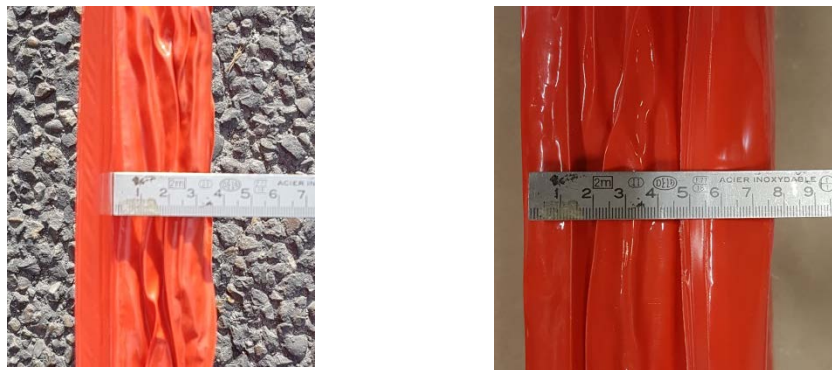
Picture 3: detail Firetight® specimen, left vacuumed, right recuperated
